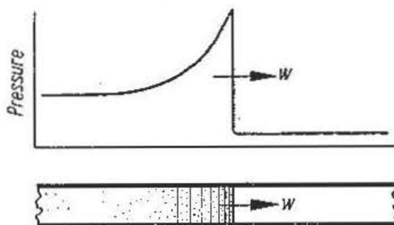
Fig. 5. Pressure distribution in tube *b* of Fig. 4
