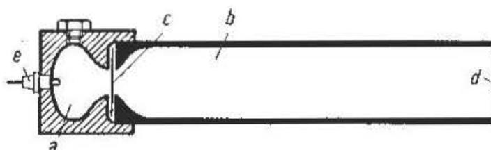
Fig. 4. Ignition device for a single shock wave
