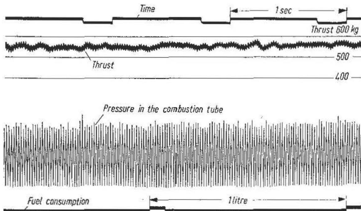
Fig. 20. Oscillogram of the 510 mm diameter Schmidtrohr
