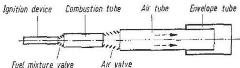
*Fig. 15. Tube with additional air*
