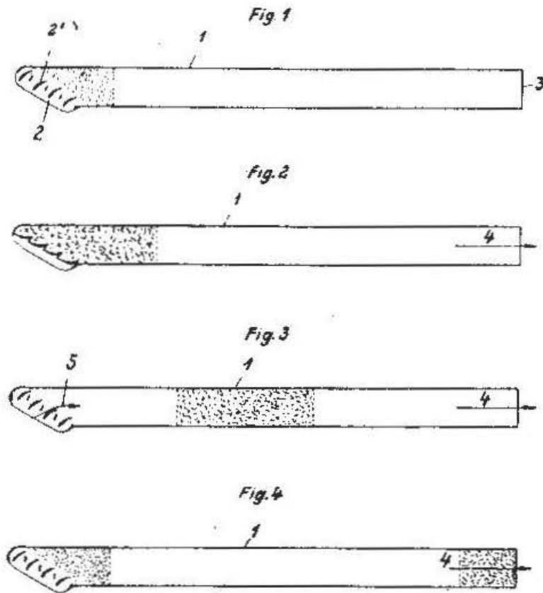
Fig. 2. Method of operation of the Schmidtrohr
