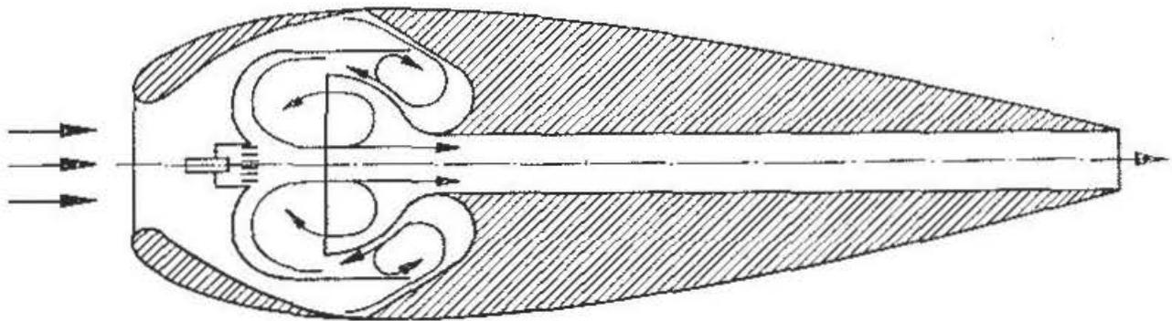
Fig. 3. Second model of the pulse jet with air intake at front
