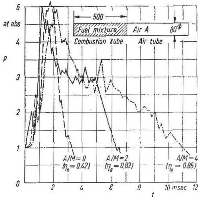
Fig. 8. Pressure in the combustion tube at different ratios  $A/M$
