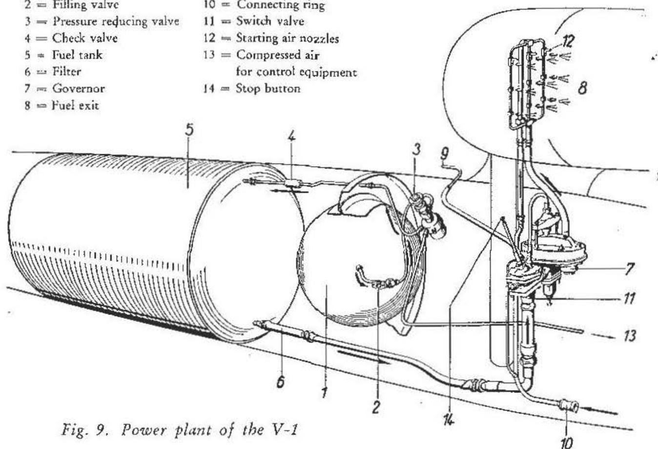
Fig. 9. Power plant of the V-1
